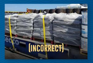
3: GROUPED CARGO LIKE PIPES, REBAR OR LUMBER SHOULD BE SECURED TOGETHER AS BUNDLES & NOT HAVE PALLETS STACKED ON THEM UNLESS ON A FIRM FOUNDATION. BAGGED LUMBER, PVC & SLICK OR LOOSE CARGO SHOULD BE BANDED TOGETHER. MULTI-LEVEL GROUPED LOADS SHOULD BE STRAPPED & SECURED AT EVERY LEVEL.
