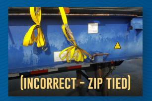
8: TURNBUCKLES AND SHACKLES SHOULD BE SECURED SO THEY DO NOT SPIN OPEN YET BE ACCESSIBLE FOR TIGHTENING WHEN NEEDED.
