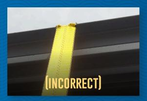
7: CHAFING GEAR / EDGE PROTECTORS MUST BE USED ON EVERY SHARP EDGE TO PROTECT STRAPS FROM CUTTING IN TRANSIT.
